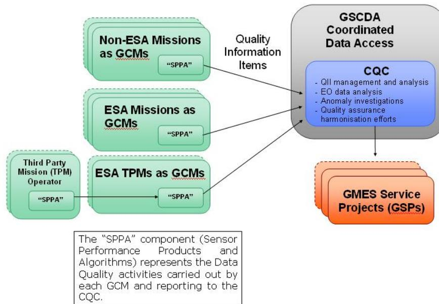
Figure 2: CQC System between GCM and GSP.
