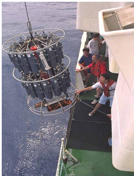
Fig. 3 : CTD probe equipped with a rosette of water bottle to sample bio-chemical parameters.
